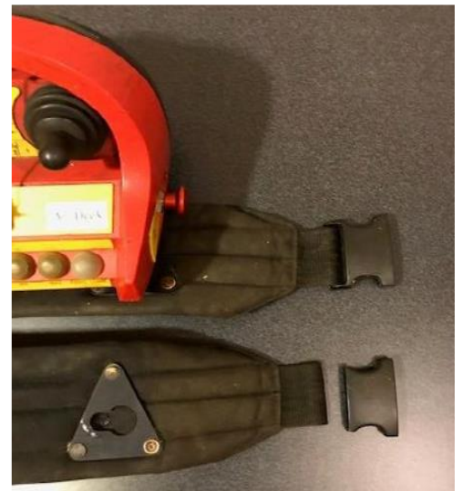
Upper: undamaged belt buckle Lower: belt buckle post-incident
