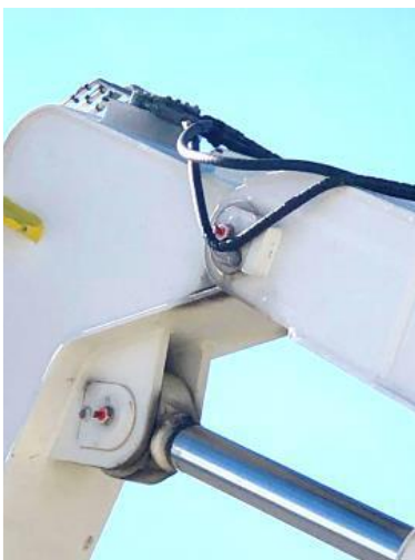
Hydraulic hose caught on the protruding grease fitting
