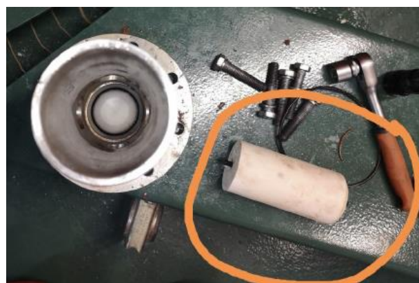
Figure 4 – Blocked Guide Tube Float
