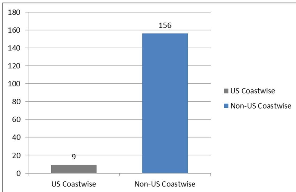
Figure 3 – Worldwide breakdown of deepwater capable light and medium construction vessels (>100T crane capacity; >1000m wire)
