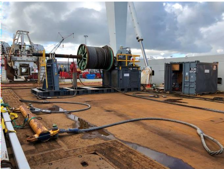
Back deck - 64mm wire rope slings connected to the spreader beam
