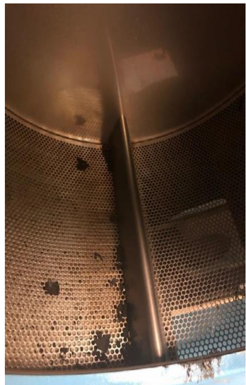
Inside tumble dryer (Dust from smouldering laundry can be seen inside)
