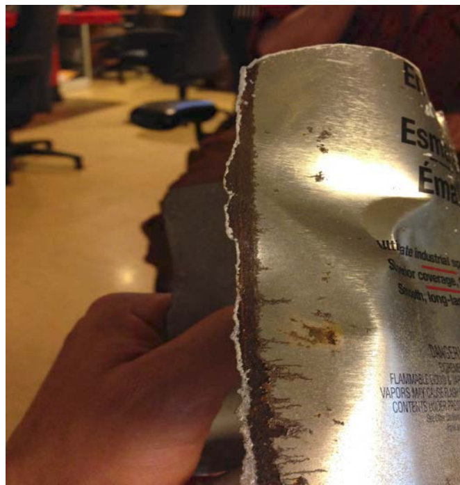
Figure 2: Ruptured aerosol can showing evidence of corrosion along seam
