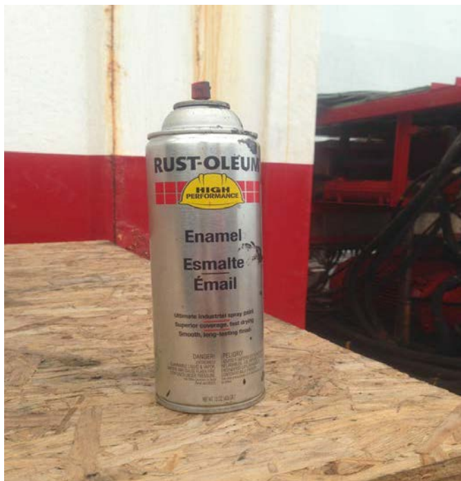
Figure 1: Aerosol Spray Paint can from same batch as ruptured can
