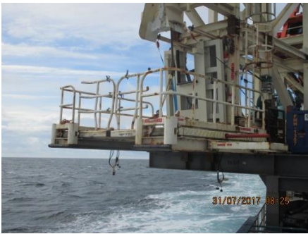
Hang off platform (HOP)
