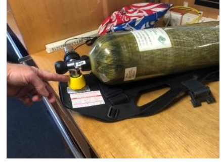
Incorrect orientation of vent valve head knob
