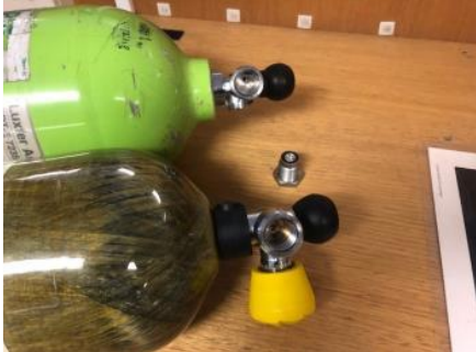
Cylinder head v/v same size thread for both 200 bar and 300 bar
