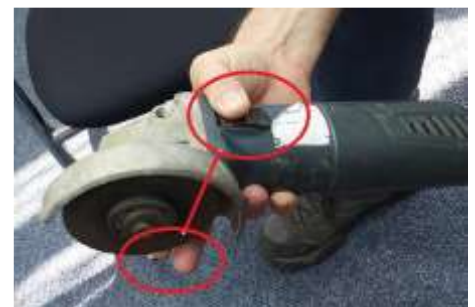
Showing INCORRECT way in which injured person picked up the grinder
