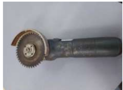
Grinder equipped with toothed saw blade, no handle and no paddle switch
