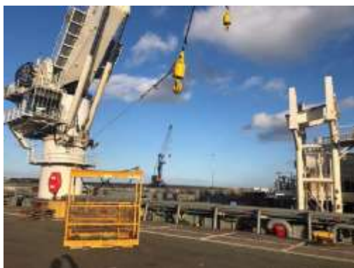
Main crane and boom rest
