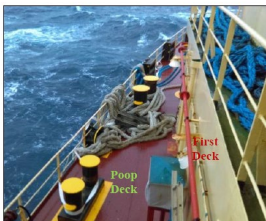
Figure 4: Situation on starboard side, two ropes secured to the railings of the poop deck, while the end of one of the ropes was hauled onto the first deck
