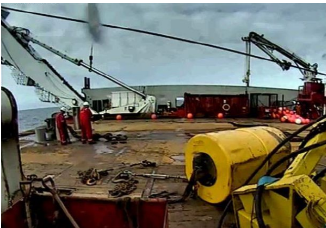
Deck crew immediately before tugger wire snaps (10:23 54'')
