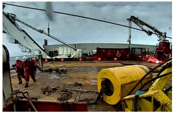
Deck crew getting out of the line of fire as tugger wire snaps (10:23 57'')
