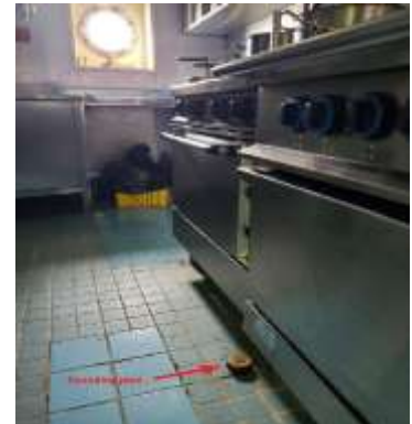
Location of sounding pipe cap
