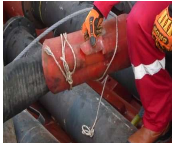
Showing point where saddle broke and sling was connected
