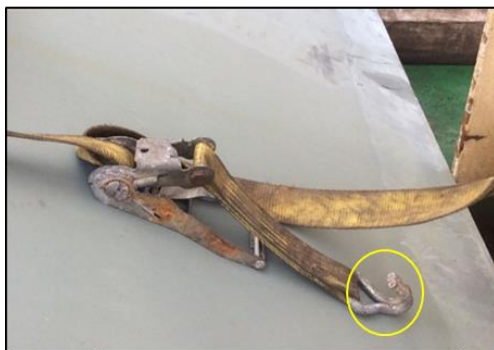
Figure #3: illustration of the ratchet strap hook that came free from the stanchion
