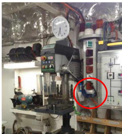
Fig. 1 Blue goggles stored unprotected
