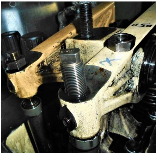
showing rocker arm adjusting screw with locking nut removed / dismantled
