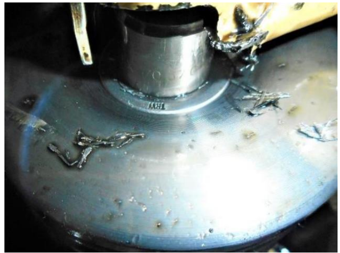
showing partial destruction of the exhaust valve tappet tip, showing also the valve roto cap
