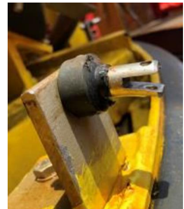
A failed latch
