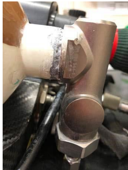
Excessive Corrosion at Cylinder Neck
