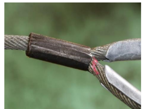
Fig. 3 Fitting is deformed with “ridges” of extra material present from over-crimping
