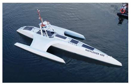
Externally the Mayflower appears a be a normal, though very modern, vessel. A trimaran design with a central hull flanked, on either side, by an outrigger. At 15m long and 6.2m wide, constructed with aluminium and composite material, the vessel weighs around 5 tonnes.
