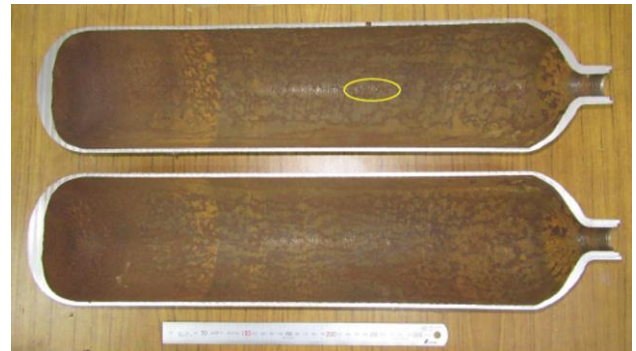
Internal surface of cylinder, showing corrosion over entire surface. Leak location circled.
