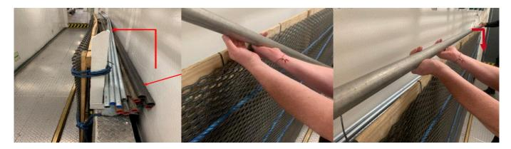
He was removing a brass bar (3m long, 47kg weight, 46 mm dia.) from the storage rack. The brass bar was lying behind a wooden frame and behind two pieces of expanded metal mesh sheets. Working alone, the injured person lifted the bar in stages to remove it from its storage. He first lifted the forward end of the bar which suddenly slipped, forcing his left hand downwards and against sharp edges on the steel wire mesh which, ripping into the skin under the weight of the bar, caused the injury.
