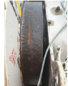
Brake band after descaling
