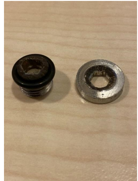
The two pieces of the failed blanking plug
