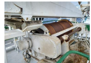
Winch unit being cleaned
