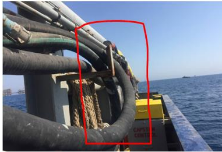
Stowage of hoses in coiled position due to long lengths
