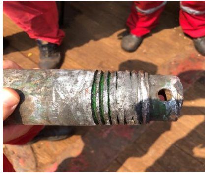
Pictures of damaged shackle nut and pin – shackle nut located STB side of winch near walkway and shackle pin found at the back of the winch. (Clear indication the shackle was side loaded)
