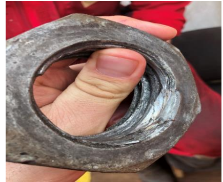
Pictures of damaged shackle nut and pin – shackle nut located STB side of winch near walkway and shackle pin found at the back of the winch. (Clear indication the shackle was side loaded)
