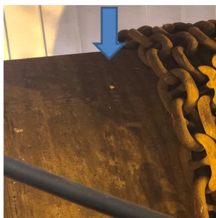
Breaking point location of shackle on drum
