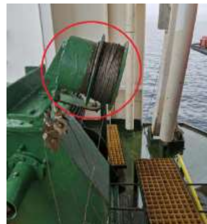
Brake release wire drum overpainted
