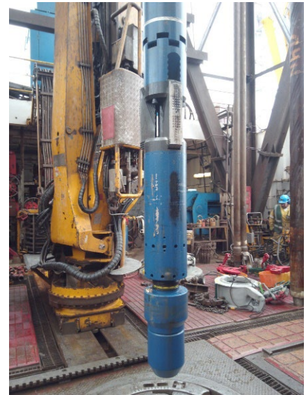
A drill-pipe deployed anchor
