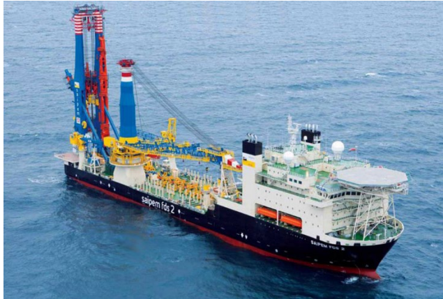
Saipem “FDS2” J Lay vessel with 2000T of vertical pipe tension capability.
