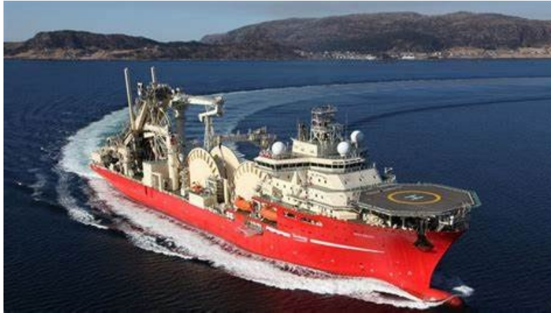
TechnipFMC “Deep Energy” Reel Lay vessel with 5600T of pipe product storage capacity
