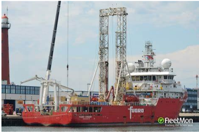
Fugro Voyager, 270ft long DP2 vessel fitted with 10,000ft water depth heave compensated seabed coring tower
