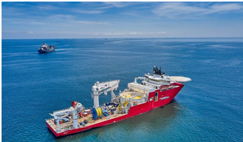
Aker “Connector” flexlay vessel with 7000T of storage.
