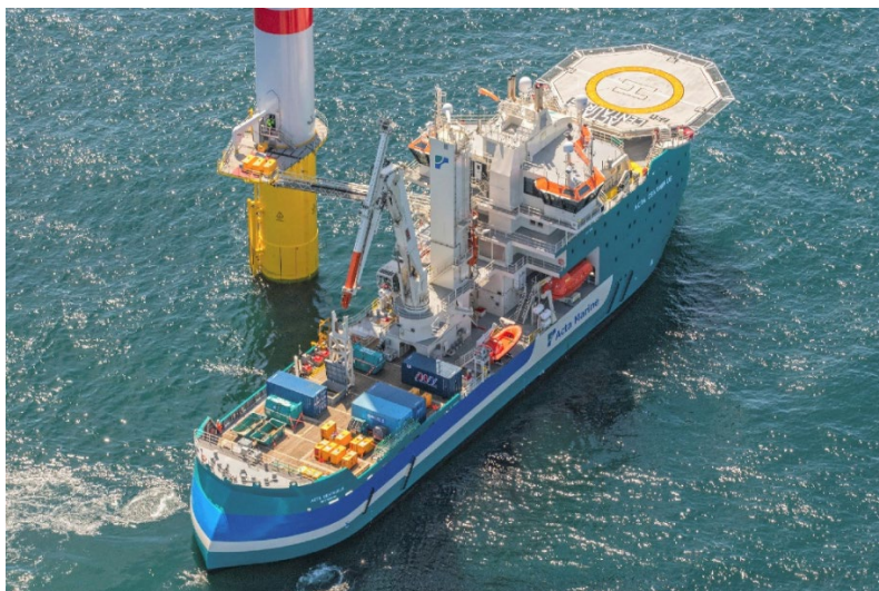
SOV transferring workers and equipment to offshore wind turbine.
