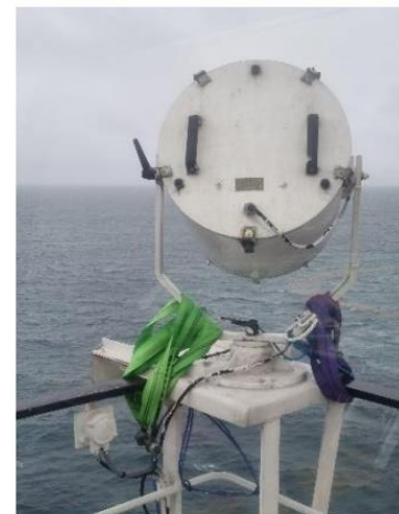
Remaining Searchlight with Additional Securing
