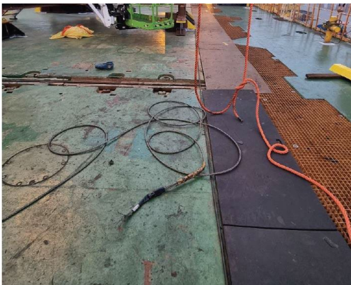
Broken messenger & auxiliary hoist wire
