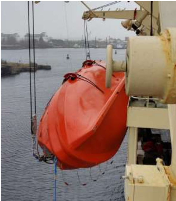
Lifeboat listing more than 90 degrees w/crew inside
