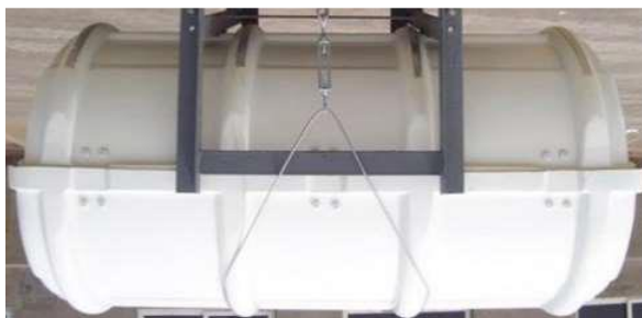
Suggested lashing arrangement using wire lash strap
