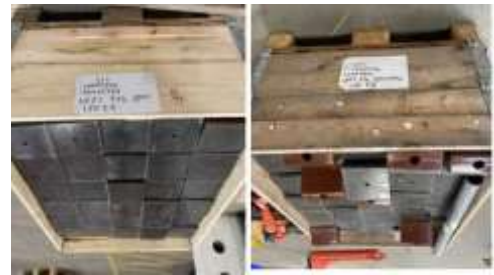
Post Incident #2 - showing appropriate wooden crates on pallets to take the load
