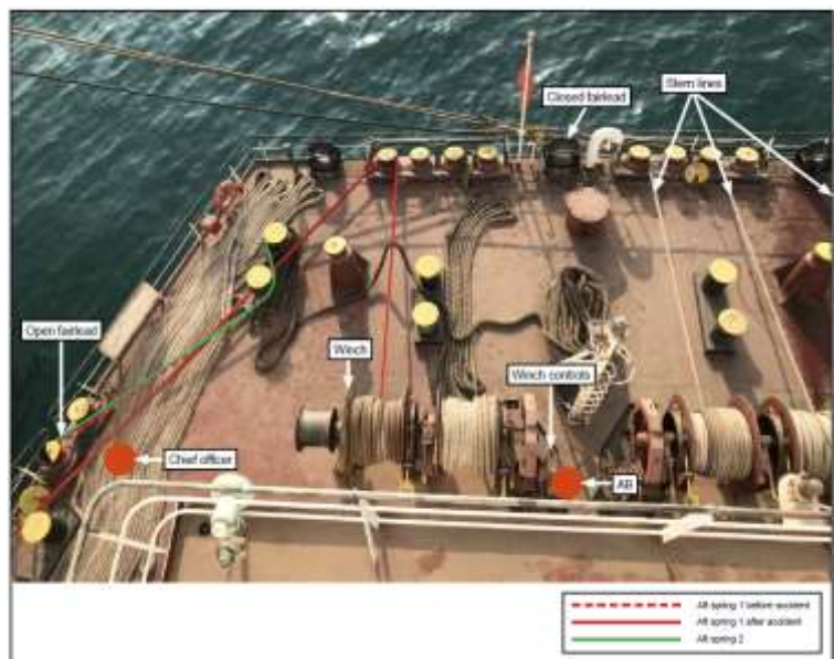
Showing mooring arrangement (dotted line indicates position of aft spring 1 before the accident)
