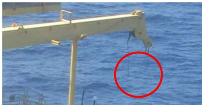
Figure 2 – Crane missing main block and auxiliary ball
