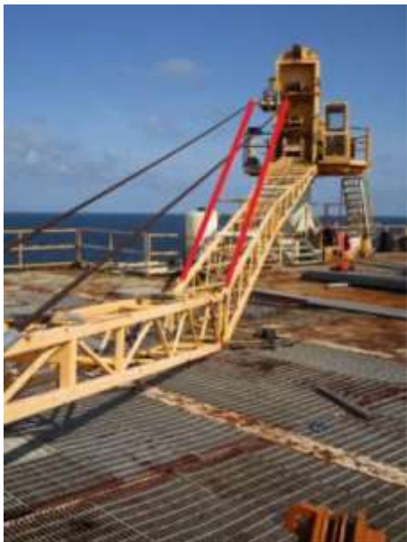
Figure 1 – Example of how mid-section should have been rigged
