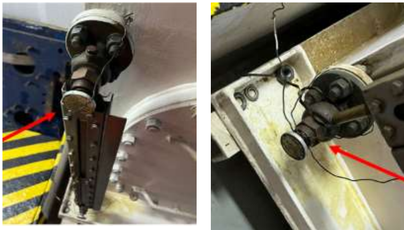
Top and bottom side of sight closing devices blocked by wire
