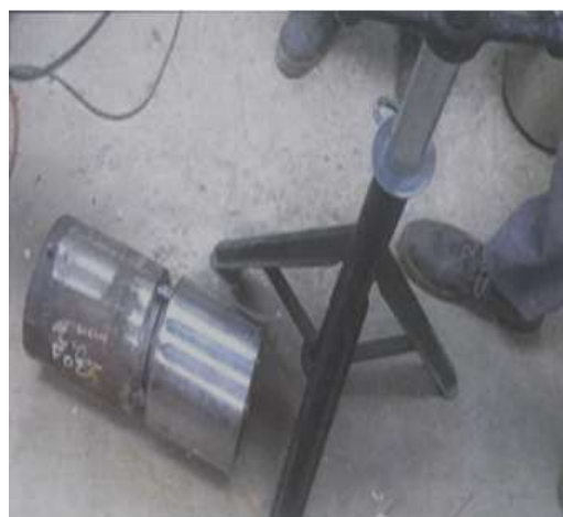
Previous Incident - Dropped welding coupon from support single stand
