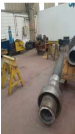
Dropped pipe from pipe supports
