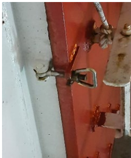
Unable to release one butterfly nut
