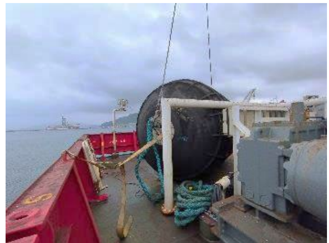
Cargo strap sea fastening still attached to Yokohama fender
