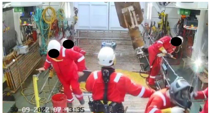
Showing A&R head ejected due to pressure
