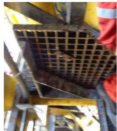
(Right) Intact manhole door raised, showing bracket in upright position. The dropped object bracket was in similar position due to previous unreported incident.
