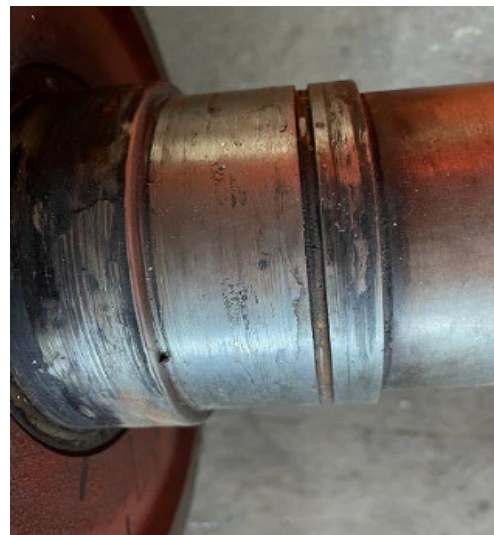
Rotor of Shaft generator/ failed bearing part caused overheating and smoke
