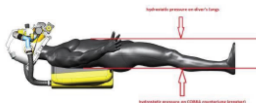
Figure 11 - Diver Face Up, Easy Inhale, Harder Exhale
