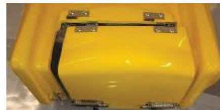
Figure 2 - Incorrect hinges and fitted upside down
