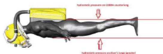
Figure 10 - Diver Face Down, Easy Exhale, Harder Inhale
