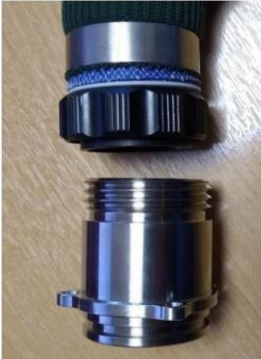
Figure 1 - Backpack Connector and Hose End
