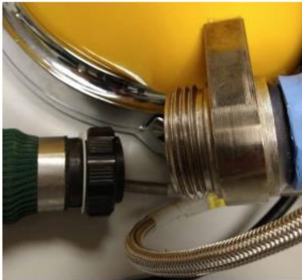
Figure 3 - Helmet Inhale Connector and Hose End
