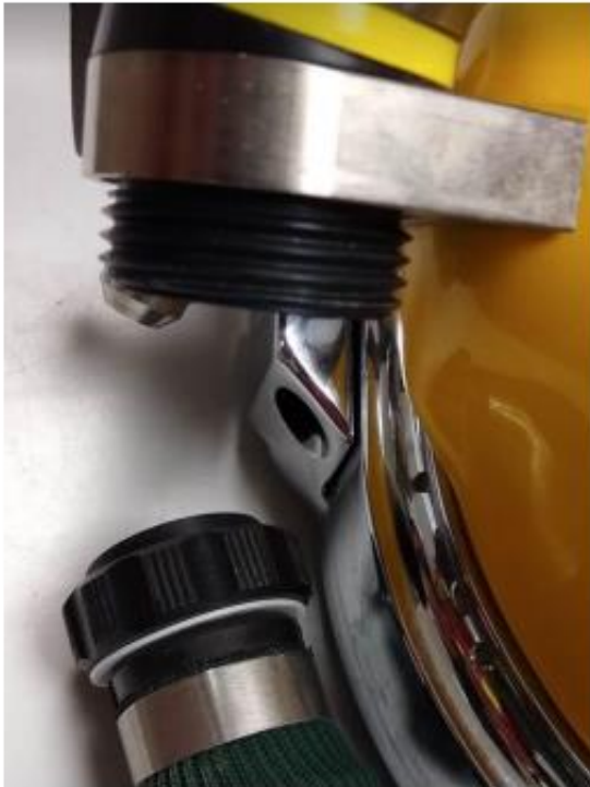
Figure 5 - Helmet Exhale Connector and Hose End
