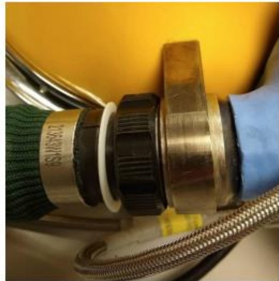
Figure 4 - Helmet Inhale Connection Correctly Made Up (no thread visible)
