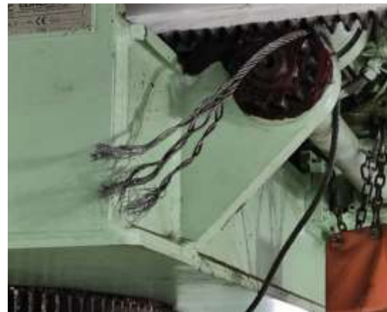
Left: cylinder liner after wire parted. Above: parted hoisting wire
