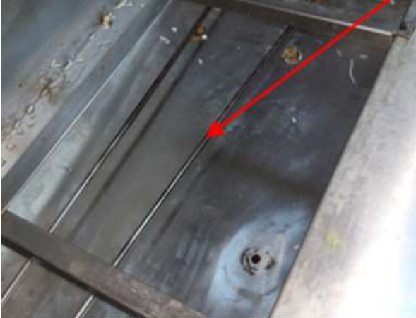
Showing earth fault of the electrical heating element
