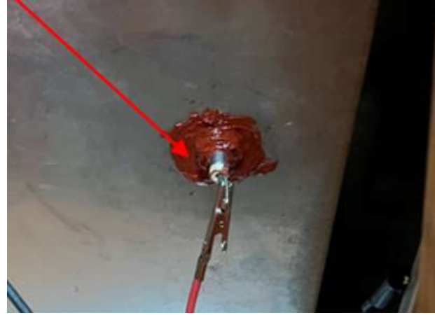
Showing earth fault of the electrical heating element
