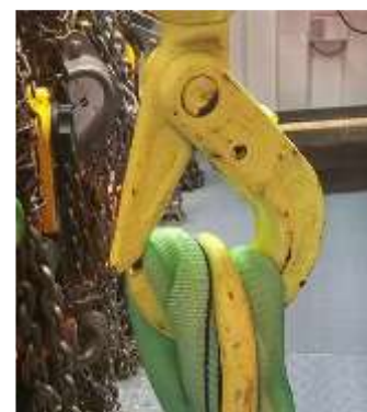
Sling preventing proper closing of the hook
