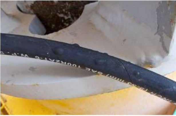
Incompatible hydraulic hose blistered during use
