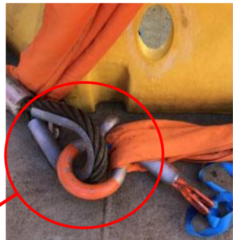
55Te ROV shackle and wire sling
