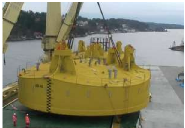
Jack-up rig leg “spud can” removed for maintenance (Image for illustrative purposes only)
