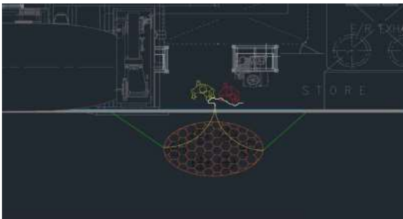
Sketch showing position of fender, the webbing straps and short hauling line
