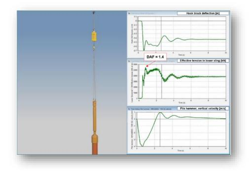
Figure 28 – Pile run with damping
