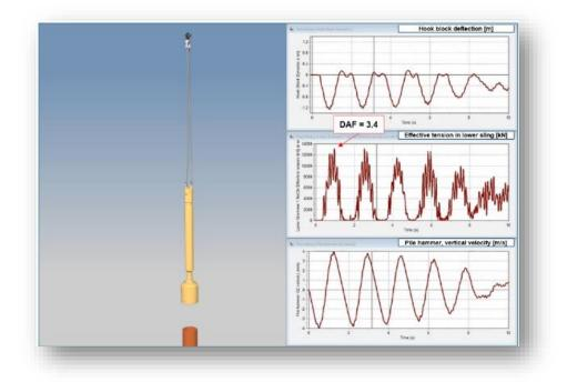
Figure 27 – Pile run; no damping
