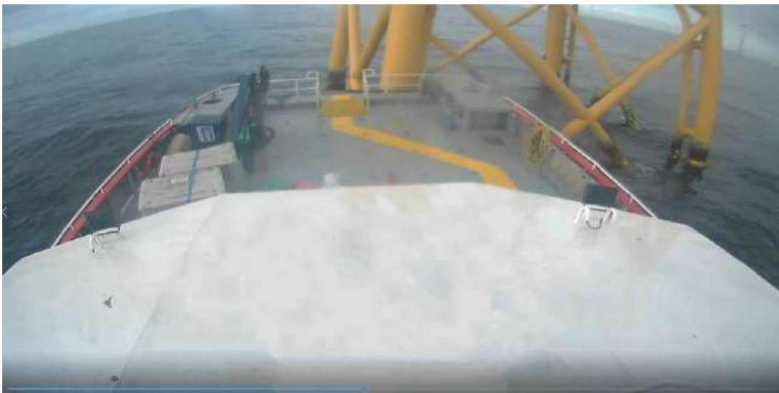
The moment the workboat bow collided with the wind turbine tower platform
