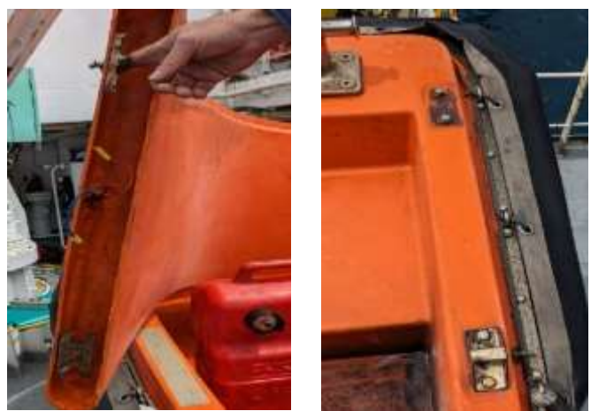
The corroded bracket on the frame and FRC
