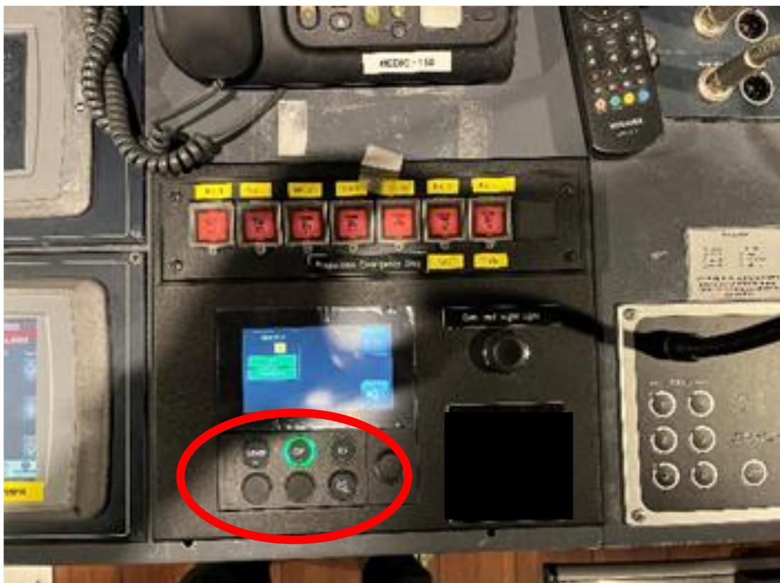
Figure 3 – Typical mode change button arrangement
