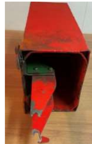
Failed/fatigued attachments points
